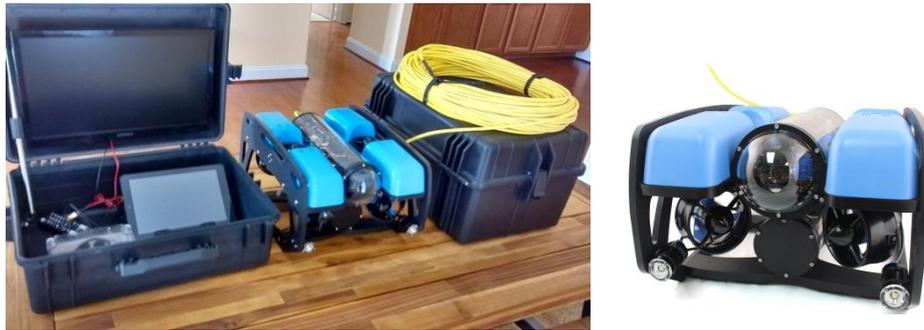
**Figure 2.** A Remotely Operated Underwater Vehicle (ROUV) used to underwater inspections, by the International Hellenic University [15].
